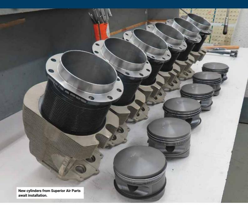
Once these steps are complete, the cylinders are prepped for installation. Staiano ordered new Superior Air Parts cylinders with matching piston weights. This is a very good choice, and not only for the performance of the cylinders. There is also a bonus of cost savings.
